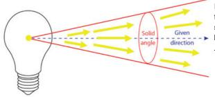
In any given direction, the luminous intensity is the flux emitted by the entire light source, per unit solid angle. The unit is lumens per steradian, better known as the candela (cd).
