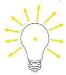
The total amount of light emitted in all directions by a light source. The unit of luminous flux is the lumen (lm).
