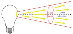
In any given direction, luminance is the luminous intensity of the source per unit of visible surface. The unit is the lumen per steradian per square metre. More simply: candela per square metre (cd/m²).
