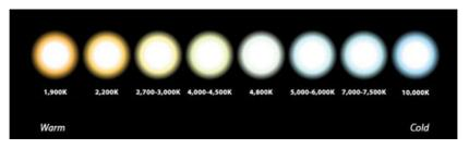
The photometric code provides several pieces of information, including the colour temperature of the LED.
