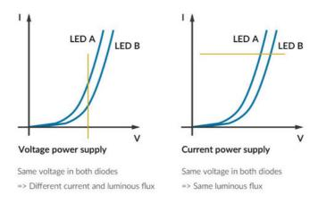
For each diode (LED) to work, approximately **3 Volts** are required at its terminals. For example, a 5-diode series requires approximately 15 Volts at its terminals. To supply regulated current at an **adequate voltage**, LEC uses an **electronic module called a driver**.
