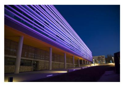
Another striking example is the path lighting, where our 6430 terminals use less than 100W to illuminate 100m of disabled access.
